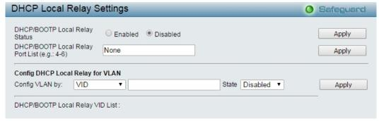
Figure 4.95 - Configuration > DHCP Local Relay Settings
