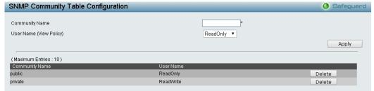
Figure 4.31 – System > SNMP Settings > SNMP Community Table
