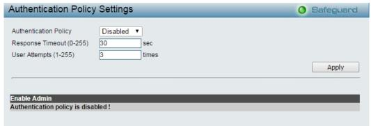
Figure 4.149 – Security > Access Authentication control > Authentication Policy Settings
