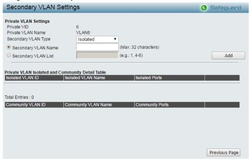
Figure 4.59 - Configuration > Private VLAN > Private VLAN Settings - Secondary VLAN Settings
