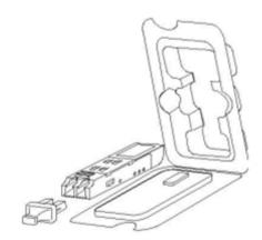
Figure 1.30 - Installing the SFP Module
